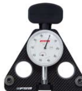
FSA Spoke Tensionmeter Gauge FSTL752-5050 • ISO and JIS certified indicator, 5 micron repeatability • Precision ball bearing spoke rollers • Easy to handle and use • Calibrated and serial numbered • Accuracy guaranteed for 10 years • Unique deflection system gives universal readings irrespective of spoke gauge • Full jeweled dial movement; shock , dust and water proof
